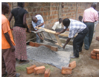
Ronnie and other participants sieving gravel for use in the Biosand water filters. Soon filters will be made in Wongonyi village.
