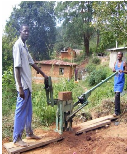
Mwandami and another youth use the brick maker to produce high quality bricks for building.
